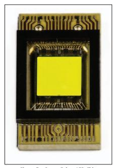
Figure 7 – Osram Eviyos LED Chip
