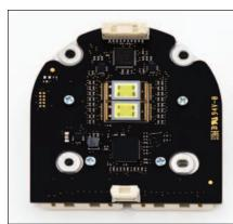
Figure 8 - Eviyos 2 Chip Layout
