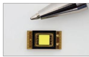
Figure 4 – Osram Eviyos LED Matrix
